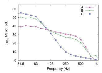
Figure 1. Pilot study noise exposure spectra.
