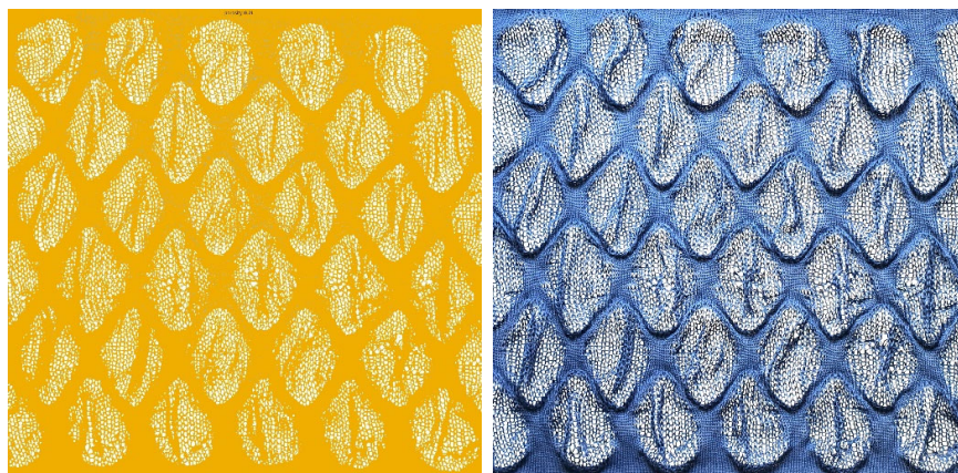
Figure 7. Porosity calculated using a script in Processing (based on pixel darkness). The calculated porosity is illustrated through colouring pixels that count as solid, here represented in yellow.
