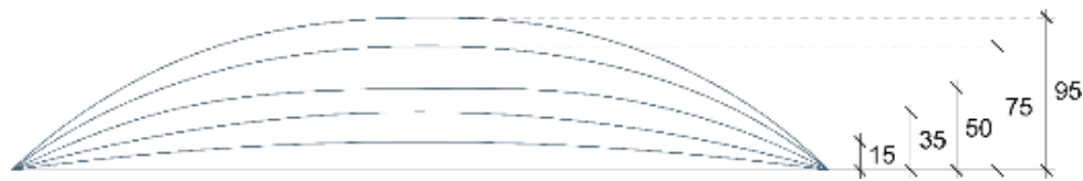
Figure 28. Estimated deformation shape of the knitted model drop-stitch 10%, based on the positions of the centre of the ellipses on the third row from the top at the different windspeeds from 0 to 15 m/s, in photos from wind-tunnel tests. The values represent distances in millimetres.
